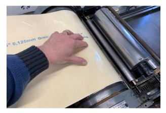
Roll the press forward in trip, keeping the tympan and packing pressed firmly against the printing drum.
