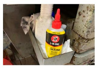
For lubricating the press mechanisms, we use the silicone 3-in-1 oil. It is a lighter weight oil, but has protective properties.
