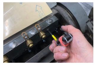
Loosen the Allen-headed bolts on the gripper plate with the Allen set from the tool wall. The necessary key is marked yellow.
