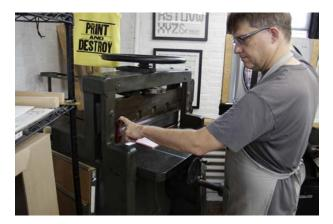
Make sure you have control of the cutter handle, and release the failsafe.
