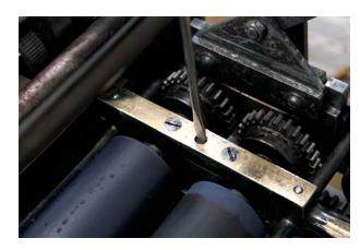
Check frequently with the roller gauge until set. Don't forget to re-tighten the set screws when done, or the rollers will shift.
