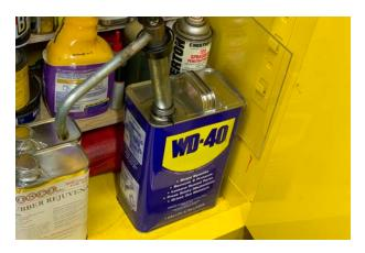
The WD-40 cannister also has a pail pump installed. Only use the designated WD-40 spray bottle, as WD-40 will dissolve other spray mechanisms.
