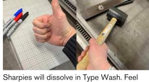
Sharpies will dissolve in Type Wash. Feel free to mark on the pressbed and Boxcar base. Also, if the Handy Lockup Bar gets stuck, use the rubber mallet, not the hammer.
