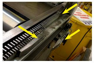
Oil the holding lever and the parts of the printing track near the top of the press.
