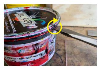
For the large 1kg vacu-seal cans, use the big screwdriver on the tool wall, and twist, don't pry the top off.
