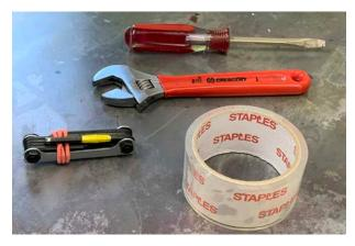
Tools you will need: the crescent wrench and small screwdriver from the tool board, and some packing tape. To change the tympan, use the folding Allen key set.
