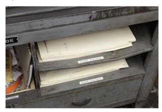
Packing comes in 0.005" and 0.008" thicknesses, located on the right-hand press shelves. The No 4 is a 0.040" press; be sure to include 0.004" for the tympan.
