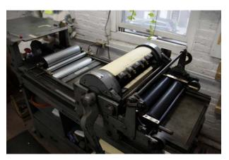
To adjust, remove the oscillating roller and place at head of press. Keep the form rollers down for constant checking.
