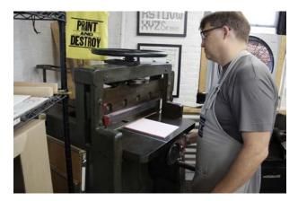
Crank the backstop into position for the appropriate cutting depth.
