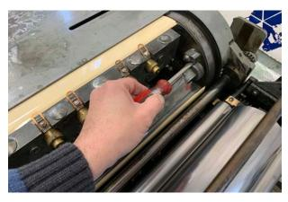
Pop the ratchet pawl on the tympan bar with the screwdriver. Do NOT unscrew the bolt. This releases the toothed ratchet wheel.
