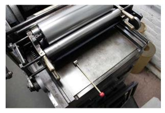
In trip, crank the print head to the end of the press. Lower the roller assembly. Use the roller gauge curved side up.
