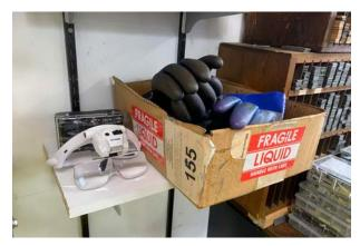
Use gloves whenever you use solvent. Also note the magnifying visor with a box of interchangable lenses – great for working with small adjustments.
