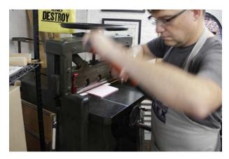
Cut with an even, controlled stroke. For soft, cottony papers, you may need to slowly rock the blade down through the stack, a quarter inch at a time.
