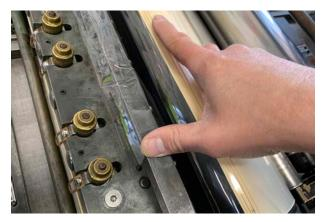
And secure the tympan end with the packing tape.
