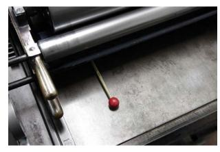
The roller gauge should gently slip underneath the rollers with a small amount of resistance. It should feel equal on all rollers.
