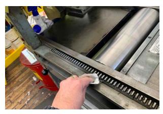
Crank the printing head forward in trip to lubricate the head of the rail as well.
