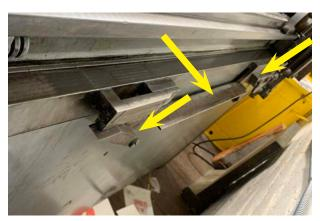
Also oil the levers and portions of the track near the bottom of the press.
