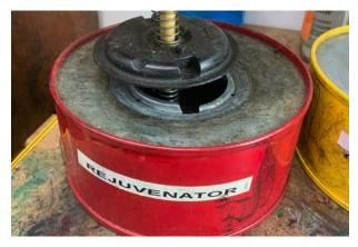
The Type Wash dispenser simply unscrews. For Rubber Rejuventor or Ultimate Orange, align tabs and pull off (shown here.)
