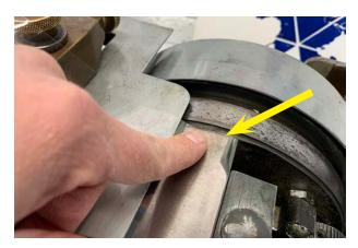
Make sure the tympan is centered and does not extend beyond the grooves in the printing drum.
