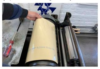
Crank the press forward slightly in trip and draw out the tympan and packing paper. You may need to tug a little to release the tape.
