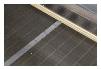
The distance from the blade forward is measured by the integral ruler on the cutter bed.
