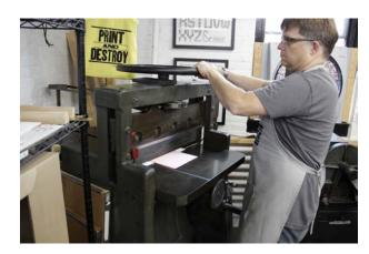
Loosen the clamp wheel to release the paper stack from the clamp.
