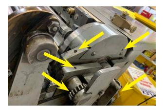
More oil: in the corresponding oil holes on the far side of the press; the bearings and gears for the print head mechanism, and the gripper plate mechanism.
