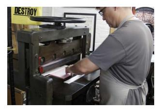
Place scrap paper above the paper stack to take the clamp pressure, and below the stack to allow the blade to cut cleanly through the stack.
