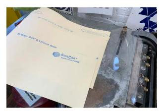
Pull out the packing sheets and add/remove sheets to modify the impression. More packing means more pressure on the form.
