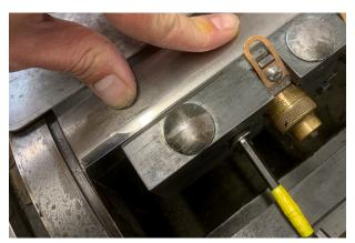
Hold the tympan in place while you tighten the Allen bolts on the gripper plate.
