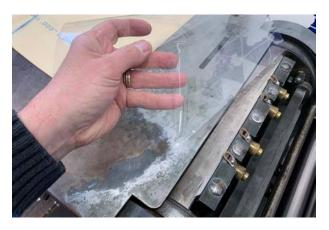
Pull the old tympan from the gripper plate, reserving the packing. Discard the old tympan in the trash.
