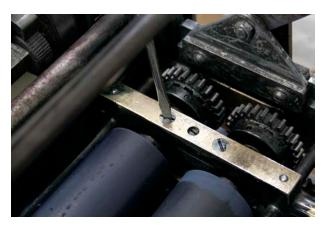
Loosen the set screws first, then adjust the rollers, using fractional turns. Remember: LEFT=LOWER, RIGHT=RAISE.
