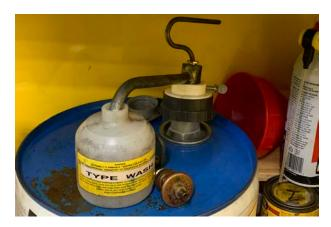
The Type Wash is in a 5 gallon pail, with a pail pump for easy dispensing. The Type Wash dispenser will fill quickly, so watch out for solvent sprays when pumping.
