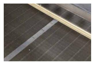
The distance from the blade forward is measured by the integral ruler on the cutter bed.
