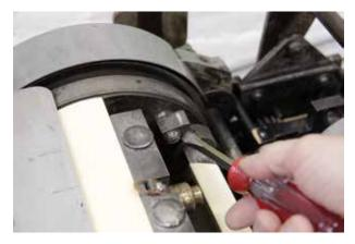
Pop the ratchet pawl on the tympan bar with the screwdriver. Do NOT unscrew the bolt. This releases the toothed ratchet wheel.
