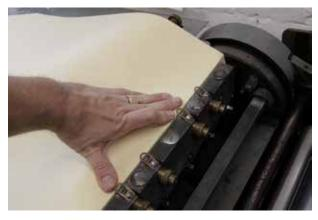
Make sure the new tympan rests snugly. It should align with the polished area of the print drum; it should not catch in the pressbed track.
