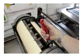
Use the Crescent wrench to tighten the tympan. *Do not overtighten – the tympan will tear!* The tympan should be drum-taut when done.
