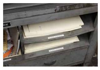
Packing comes in 0.005" and 0.008" thicknesses, located on the right-hand shelves. The No 4 is a 0.040" press; be sure to include 0.006" for the tympan.
