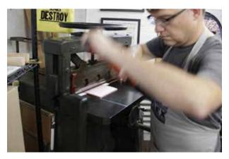
Cut with an even, controlled stroke. Do not put undue pressure on the machine.
