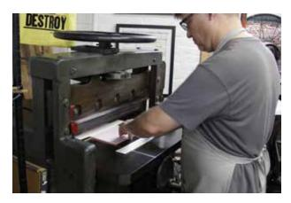
Place scrap paper above the paper stack to take the clamp pressure, and below the stack to allow the blade to cut cleanly through the stack.
