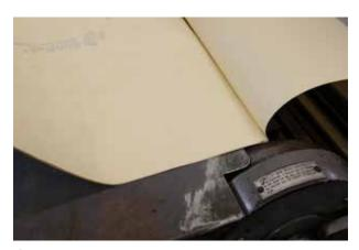
Carefully stack the packing paper under the tympan, again making sure it is aligned with the print drum.
