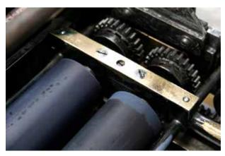
Three bolts attach to the roller frame on either end. The middle one is a set screw; the others adjust the roller height.
