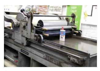
Crank the printing head forward in trip to lubricate the head of rail as well.
