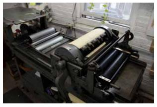
To adjust, remove the oscillating roller and place at head of press. Keep the form rollers down for constant checking.
