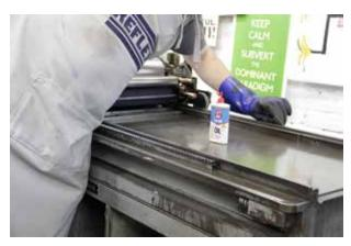
Repeat for the other side of the press – top and bottom of rail and top of bearing platform. Record the date in the log on the wall next to the end of the press.
