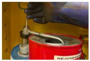
Pump carefully, being mindful of the level of solvent in the container. This is especially important with NTT Wash.
