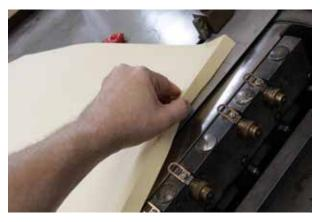
Fold the score line on the new tympan for ease of placement. Slip the folded edge into the seam between gripper plate and print drum.
