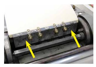
Loosen the two machine screws holding the gripper plate to the printing drum.
