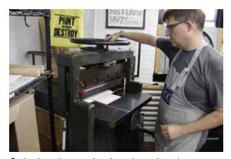
Spin the clamp wheel to drop the clamp down on the paper stack. Be sure the paper stack is secure, or else you will cut trapezoids, not rectangles.
