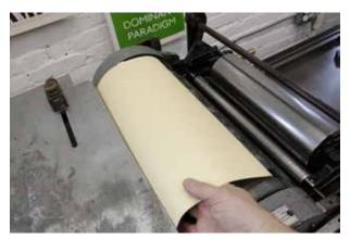
Crank the press forward slightly in trip and draw out the old tympan and packing paper.
