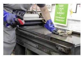
Wipe down the pressbed in its entirety, including the guide rails.
