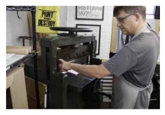
Make sure you have control of the cutter handle, and release the failsafe.
