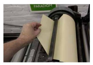
Draw the tail under the tympan bar. Make sure the packing does not come loose.
