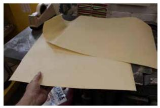
Stretch the packing and old tympan across the paper board, bringing the press back to home. Pull out the packing sheets.
