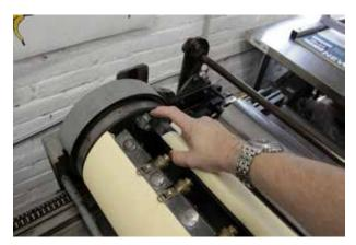
Flip the ratchet pawl on the tympan bar so gravity makes it rest against the ratchet wheel. Turn bar until finger tight.
