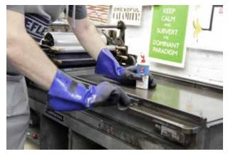
Wipe the top of the near press rail to the end of the bed. The idea is to renew the film of oil, not to saturate it with puddles.
