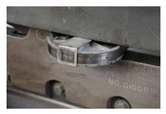
The distance behind the blade to the paper backstop is measured by the tape. It is good to  $\pm 1$  mm.
