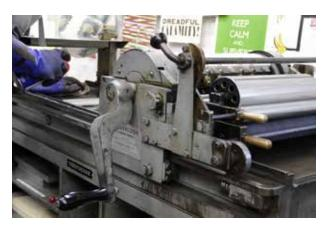
Don't forget to crank the press forward to get under the paperboard.
