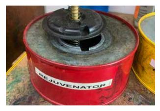
The NTT Wash dispenser simply unscrews. For Super Rubber Rejuventor or Ultimate Orange, align tabs and pull off (shown here.)
