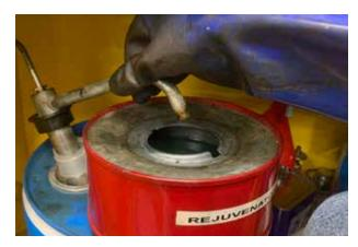
When container is full, tilt back solvent pump so that no fluid emerges from the nozzle. This is important to prevent siphoning.
