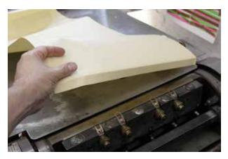
Pull the old tympan off the printing drum. Discard (or display, if interesting enough). Replace packing as needed.
