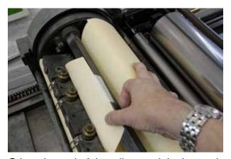
Crimp the end of the tail around the bar and begin wrapping. A piece of masking tape can help secure the tail to the bar.
