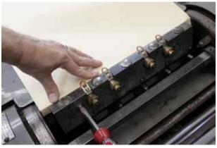
Be sure to tighten down the gripper plate machine screws firmly, or the gripper assembly can shift during printing and possibly come off.
